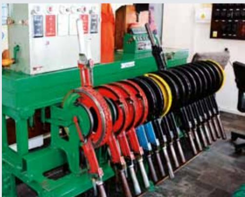
Lever frame placed on the railway signal tower St. 1
